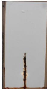
油性光油(直接塗佈銹蝕瓷漆)
