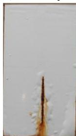
油性光油(直接塗佈銹蝕瓷漆)
